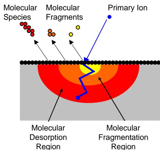
The secondary ions which desorb from the sample surface are analyzed and their mass is determined with high accuracy. As a result, elemental and molecular chemical information can be obtained on both insulating and conducting materials. TOF-SIMS allows spectroscopy for characterization of chemical composition, imaging for mapping the surface distribution of species, and depth profiling.
