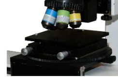
Fine Leveling Stage \pm 2^\circ or \pm 4^\circ
